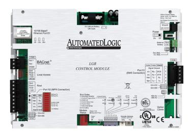
The Automated Logic® LGR router is an integral component of the WebCTRL® building automation system.
